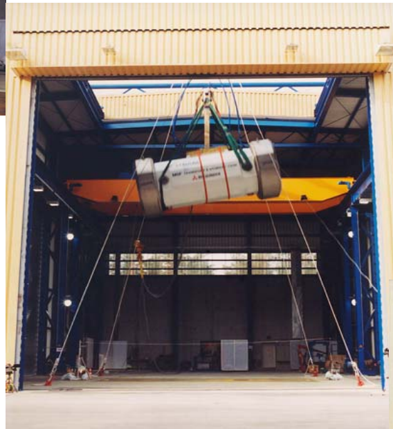
9 meter drop test of a big full scale cask for the transport and storage of nuclear waste
